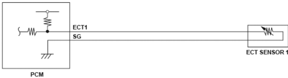
Fig. 13: Engine Coolant Temperature (ECT) Sensor 1 (High Voltage) - Circuit Diagram
