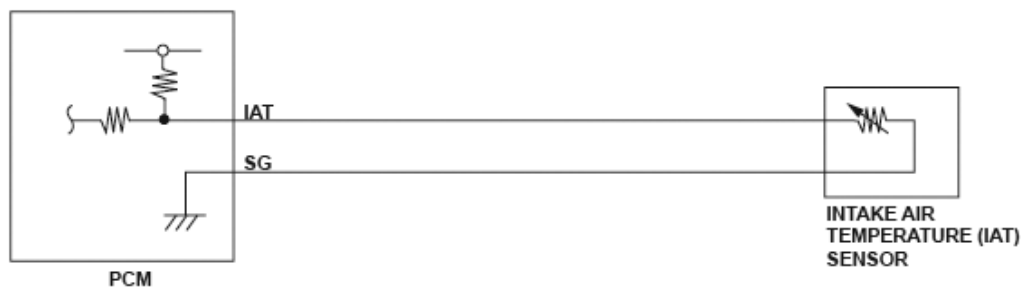
Fig. 8: Intake Air Temperature (IAT) Sensor (High Voltage) - Circuit Diagram
