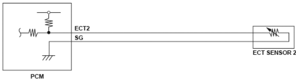
Fig. 268: Engine Coolant Temperature Sensor 2 (Low Voltage) - Circuit Diagram
