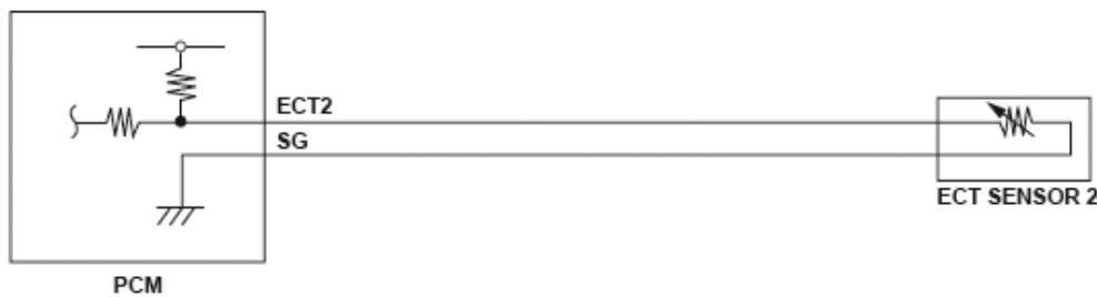
Fig. 270: Engine Coolant Temperature Sensor 2 (High Voltage) - Circuit Diagram
