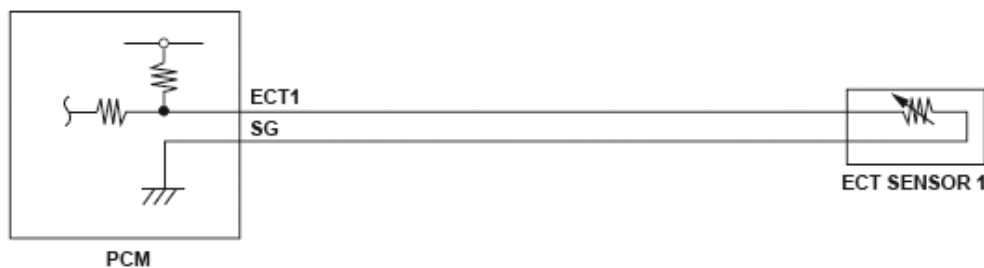
Fig. 11: Engine Coolant Temperature (ECT) Sensor 1 (Low Voltage) - Circuit Diagram
